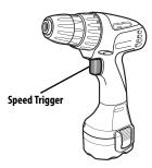
trigger. To turn the Drill Winch OFF, release the trigger. The speed is controlled by the amount of trigger depression.
